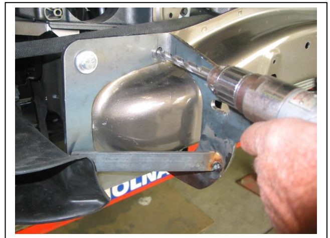
Figure 2: Drill four holes to 10mm (per side)
