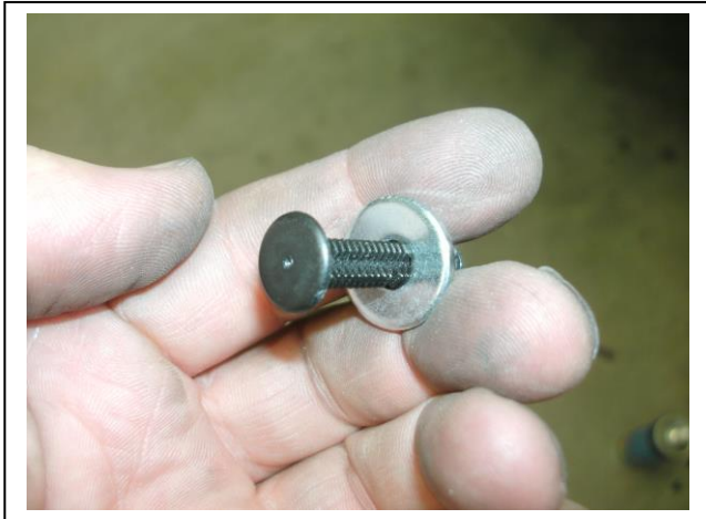
Figure 5: Place M6 washer over Christmas tree plug to enlarge size of head.
