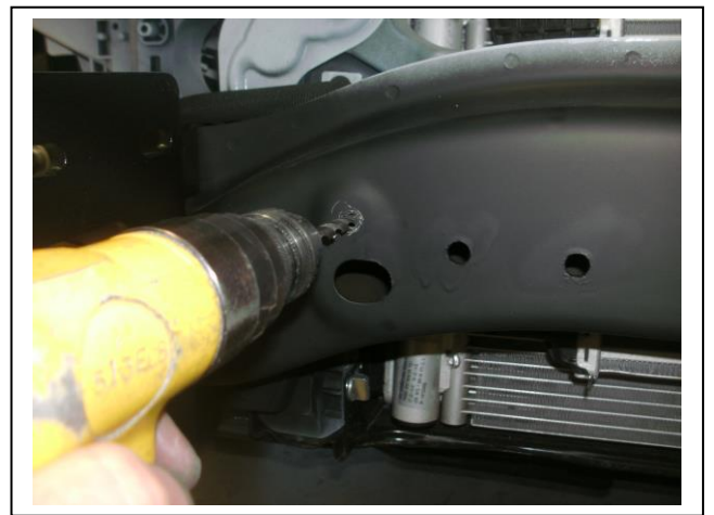
Figure 4: Enlarge one hole per side for polystyrene foam bumper support
