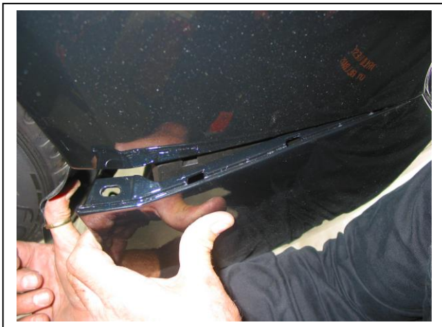
Figure 1: Pull bumper rearward and out to release.
